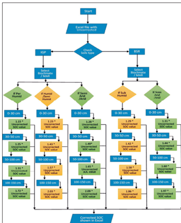
Fig. 10 : Flow chart showing the steps to correct soil organic carbon using the corrected Walkley Black Recovery Factors.
